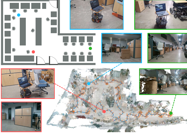
Fig. 6: Real world validation. Schematic representative map of the lab (top-left) and the resulting 3D point cloud reconstruction (roof cropped for visibility). The robot’s trajectory begins at the green starting point. The surrounding color-coded images corresponding to the green, blue, and red markers, display the robot in the environment alongside its egocentric view at that exact moment during capture, including a point cloud from the starting location.
